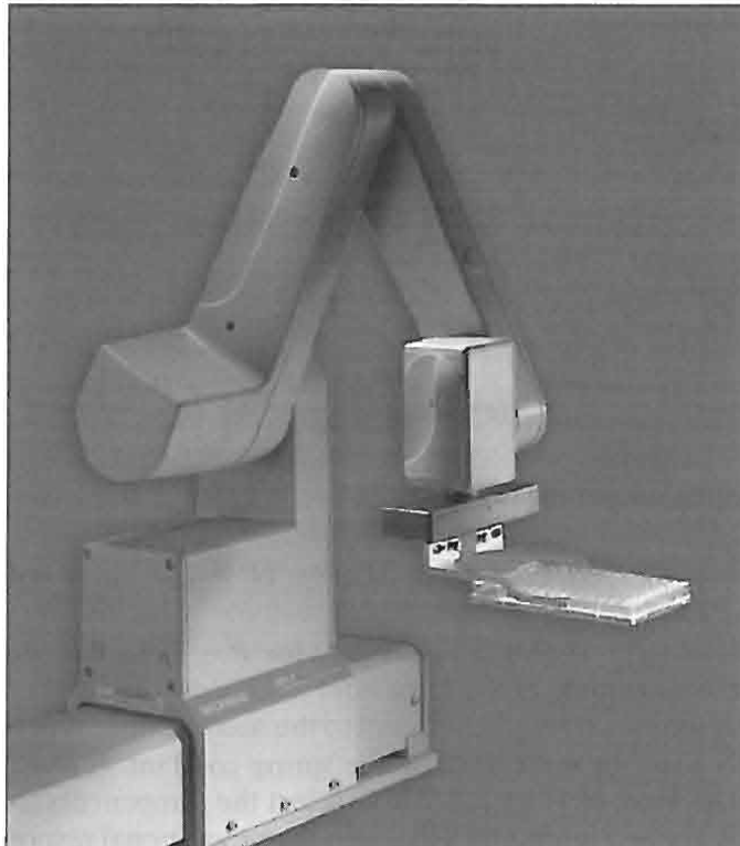
FIGURE 2.43 Laboratory robot used for sample preparation. The robot manipulates small objects, such as test tubes, and probes in and out of tight places at relatively high speeds [15]. (Photo courtesy of Beckman Coulter, Inc.)
